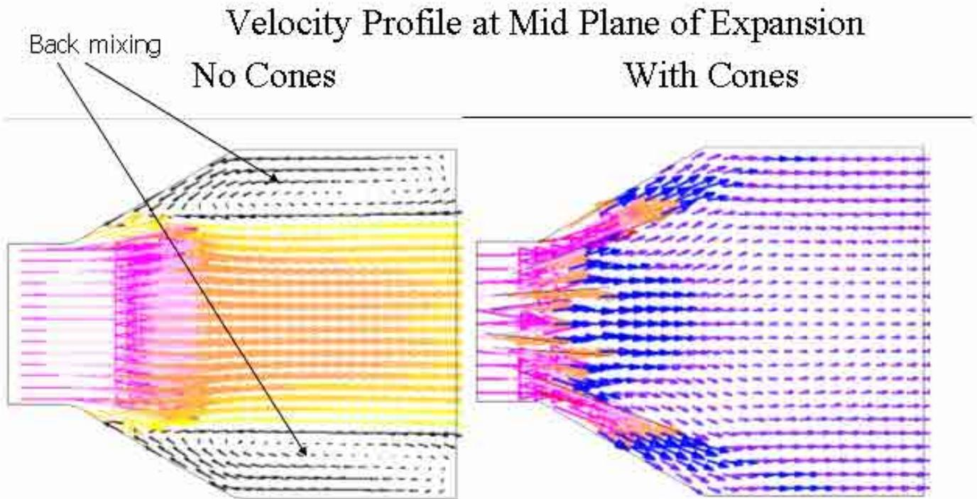
**Figure 5. Without cones in a large expansion, significant back mixing occurs with a high velocity jet in the center. With overlapping concentric cones, the velocity profile through the expansion becomes uniform.**
