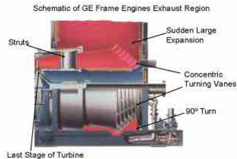
Figure 1. A Schematic of GE Frame Gas Turbine showing the exhaust gas path and areas where large pressure losses occur.
