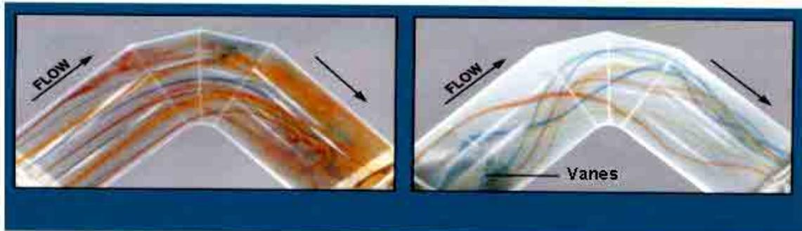
Figure 3. When water flows through an elbow, separation and turbulence occur. Using specially designed vanes to pre-rotate the fluid, the fluid negotiates the turn with all streamlines traveling in equal flow paths.
