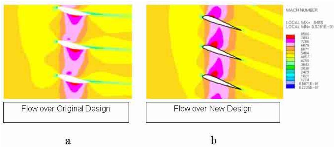
Figure 2. Differences in Flow Behavior between (a) the current strut design and (b) new strut design. The inlet conditions represent full speed full load operation. The turbulence caused by the current design leads to large pressure losses and removes the swirl that leads to large pressure losses downstream of the struts.
