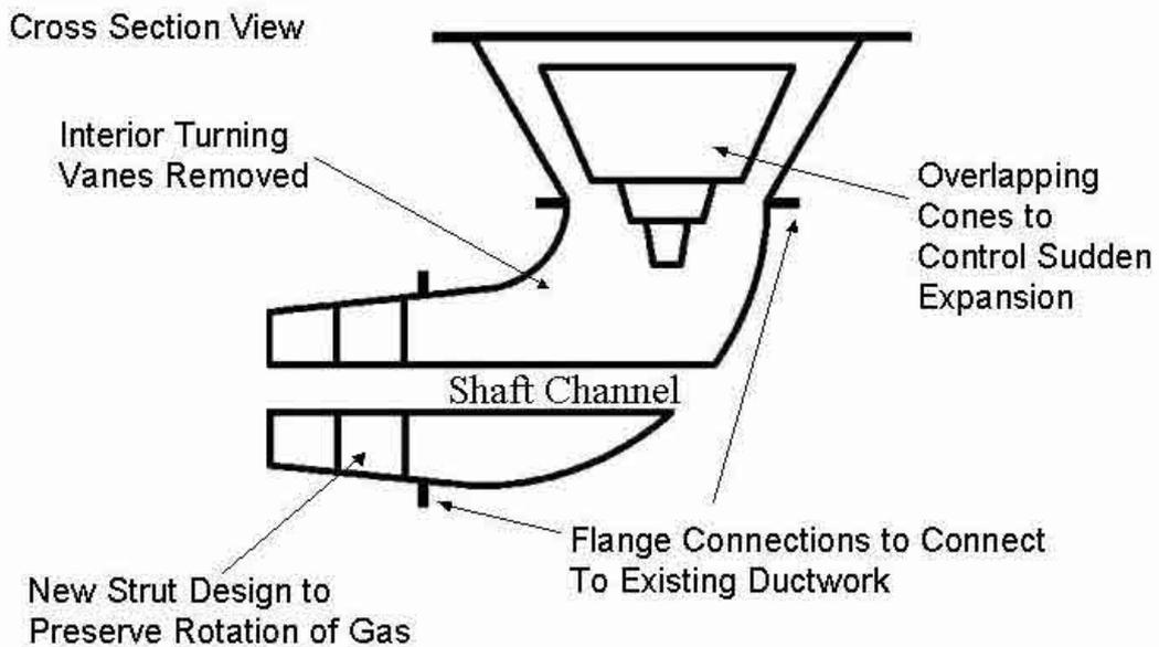
**Figure 6. This is a schematic of a new tailpipe design that fits within the current space of the old design shown in Figure 1. The struts will be modified to the new shape shown in Figure 2. Downstream of the struts the wall and turning vanes will be replaced with an elbow.**
