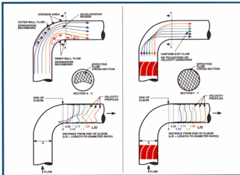
Figure 4. In a plain elbow with air flowing through, a skewed velocity profile results at the exit. With pre-rotation vanes, there is a flat velocity profile.
